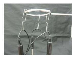
5. Place the temperature sensors into the beakers filled with water and arrange them as shown below, ensuring the sensors do not touch the bottom of the beakers.
